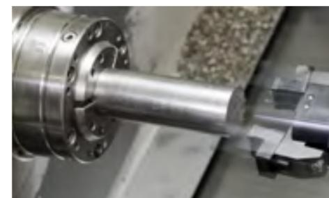
Move the bar puller in Z direction off the bar and start machining.
