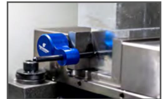
**Workpiece stopper with magnetic base**
